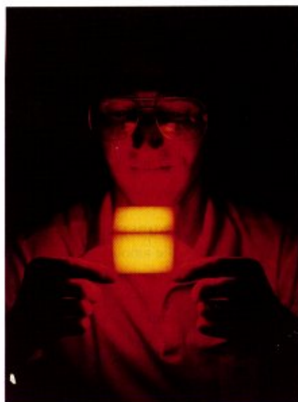
17.21 This protective tile, developed for use in the space shuttle, has extraordinary thermal properties. The extremely small thermal conductivity and small heat capacity of the material make it possible to hold the tile by its edges, even though its temperature is high enough to emit the light for this photograph.
